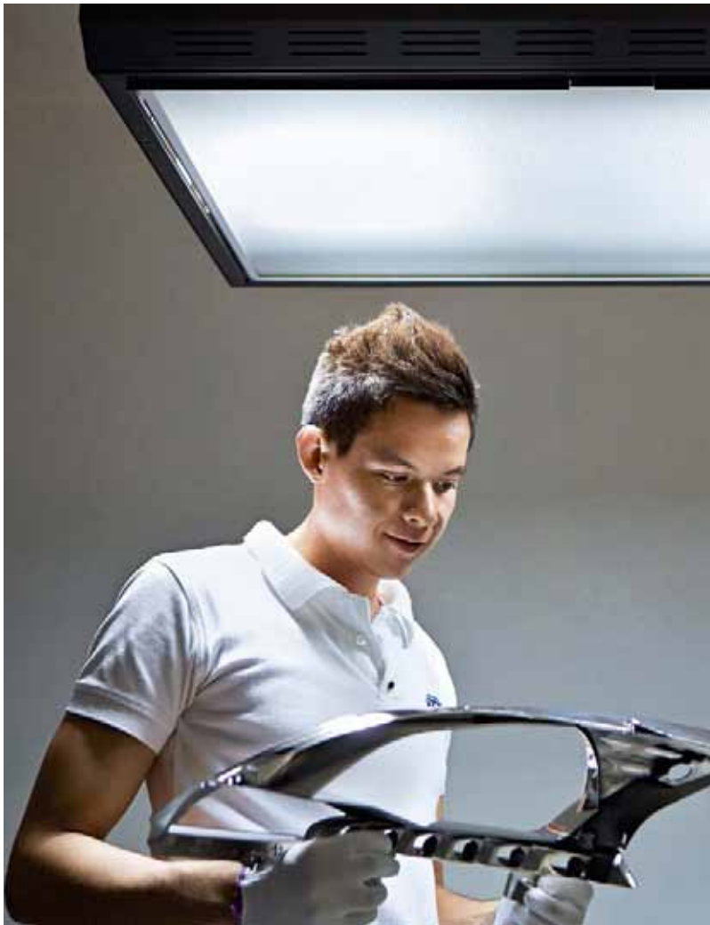
Visual quality checks on a headlamp cover frame before further processing.
